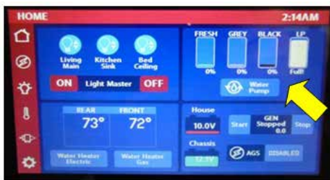
Touch Screen Tank Monitor example
