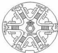
7-way trailer plug car end, rear view
