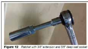
Figure 12 Ratchet with 3/8" extension and 5/8" deep well socket
