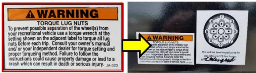
Lug nut torque pattern and warning label
