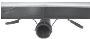
Black/Grey Tank Drain and Valves
