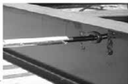
Fig. 2 - Through Frame Crank Extension w/Pin
