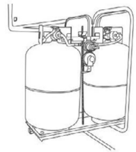
Two Propane Cylinders
