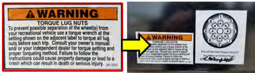
Lug nut torque pattern and warning label
