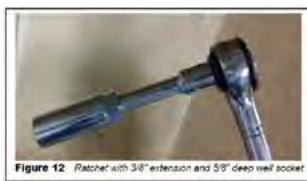
Figure 12 Ratchet with 3/8" extension and 5/8" deep well socket
