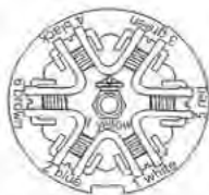
7-way trailer plug car end, rear view
