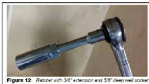
Figure 12 Ratchet with 3/8" extension and 5/8" deep well socket
