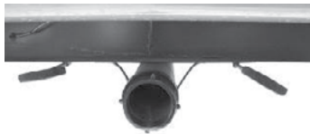
Black/Grey Tank Drain and Valves
