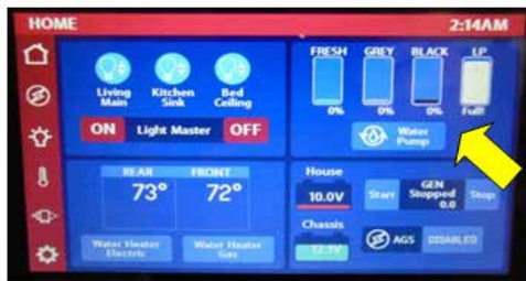
Touch Screen Tank Monitor example
