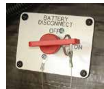
Battery Disconnect Switches
