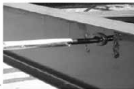
Fig. 2-Through Frame Crank Extension w/Pin
