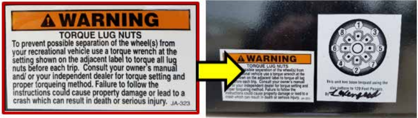
Lug nut torque pattern and warning label
