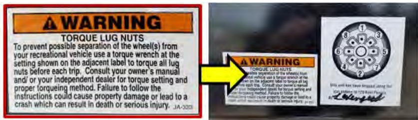
Lug nut torque pattern and warning label
