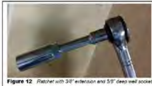
Figure 12 Ratchet with 3/8" extension and 5/8" deep well socket
