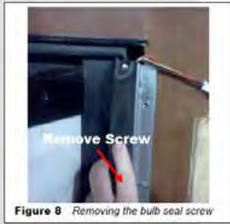
Figure 8 Removing the bulb seal screw
