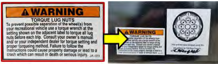
Lug nut torque pattern and warning label
