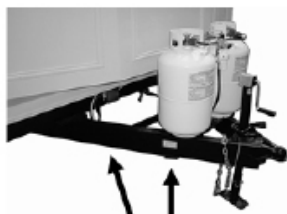
Electrical wiring & safety break-a-way switch Detachable Hitch
