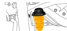
JOUNCE BUMPERS Assist during extreme road occurrences to absorb impact and dampen excess road noise
