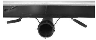
Black/Grey tank drain & valves
