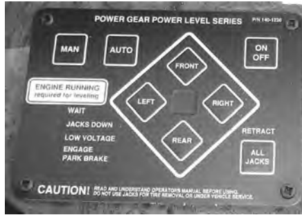
Auto Leveling Control Panel
