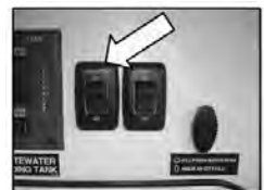
Macerator power switch
