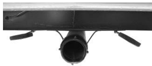
Black/Grey Tank Drain & Valves
