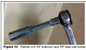
Figure 12 Ratchet with 3" extension and 5/8" deep well socket
