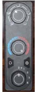
**NOTE:** When outside ambient temperatures are below approximately 40° F, the A/C compressor may cycle rapidly. Use FRESH AIR mode instead of A/C in these temperature conditions to cool the interior air temperature. For operational safety in the event of the loss of vacuum, the HVAC system is designed to discharge air through the defrost vents to provide continuous windshield defogging.
