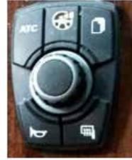
**Knob Controller:** To display the Cameras or the Navigation screen, push the knob upward and the screens on the dash will change. They will cycle through the Digital Dash, Navigation screen, and the outside Cameras. Each time you push the knob upward it will change the screen on the dash. Pushing it upward (3) times will return to the Digital Dash screen.
