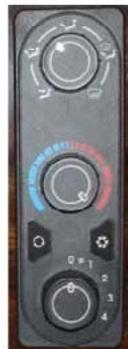
**NOTE:** When outside ambient temperatures are below approximately 40° F, the A/C compressor may cycle rapidly. Use FRESH AIR mode instead of A/C in these temperature conditions to cool the interior air temperature. For operational safety in the event of the loss of vacuum, the HVAC system is designed to discharge air through the defrost vents to provide continuous windshield defogging.
