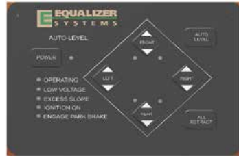
Hydraulic Control Panel
