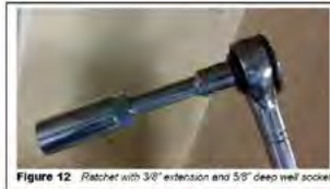
Figure 12 Ratchet with 3/8" extension and 5/8" deep well socket
