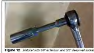
Figure 12 Ratchet with 3/8" extension and 5/8" deep well socket
