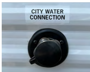
City Water Connection Example
