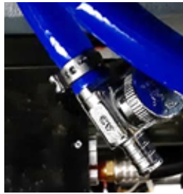
Fresh Water Drain Valve
