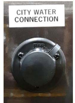
City Water Fill w/Connection Label
