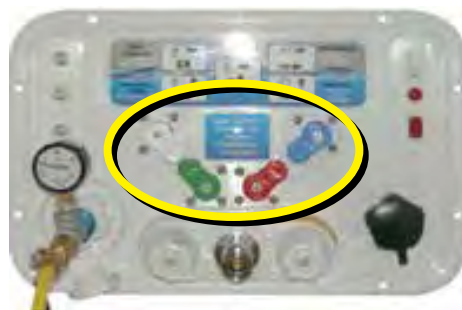
Fig 2: Set 4 Valves to 45°
