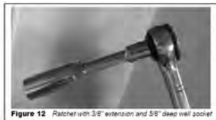
Figure 12 Ratchet with 3/8" extension and 5/8" deep well socket
