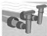
Low point drains
